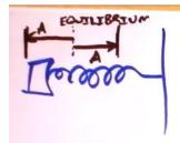
Take a look at this drawing of a spring attached to a wall on the right and mass on the left. When you leave it alone, it stays at an equilibrium position. When you pull it or push it, the distance you pull or push is giving the spring an amplitude, A.
