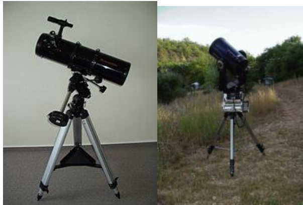
Left: Reflecting telescopes used by amateur astronomers today are similar to the one designed by Isaac Newton in the 17 th century. Right: A modern variation of the reflecting telescope, known as a ‘Schmidt–Cassegrain’ telescope.
